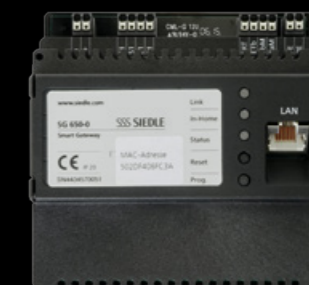
The Siedle Smart Gateway is the interface to door communication.
